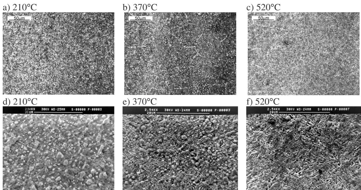
Figure 3. Microstructures of the researched steel after hardening from 900°C and heating with the velocity 0,05°C/s to different temperatures after nital etching a), b), c) light microscope, d), e), f) scanning microscope
