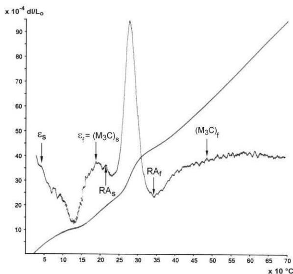
Figure 1. Dilatograms of heating with the velocity  $0.05^\circ\text{C/s}$  of a sample previously hardened from  $900^\circ\text{C}$  with the corresponding differentiation curve
