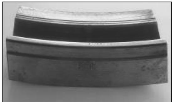
Fig. 2. Outer bearing ring test sample
