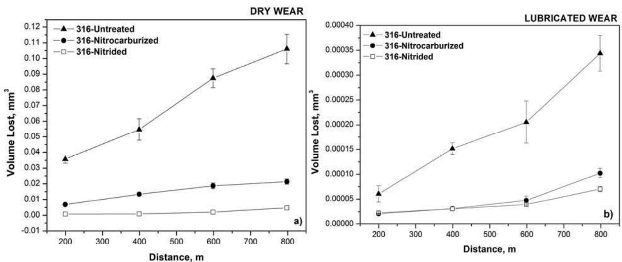
Fig. 4. Volumetric loss curves against distance for: (a) dry wear and (b) lubricated wear, of the plasma nitrided and nitrocarburized AISI 316 stainless steel
