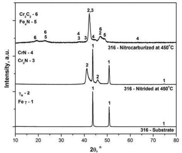
Fig. 2. X-ray diffraction patterns of untreated, nitrided and nitrocarburized AISI 316L steel
