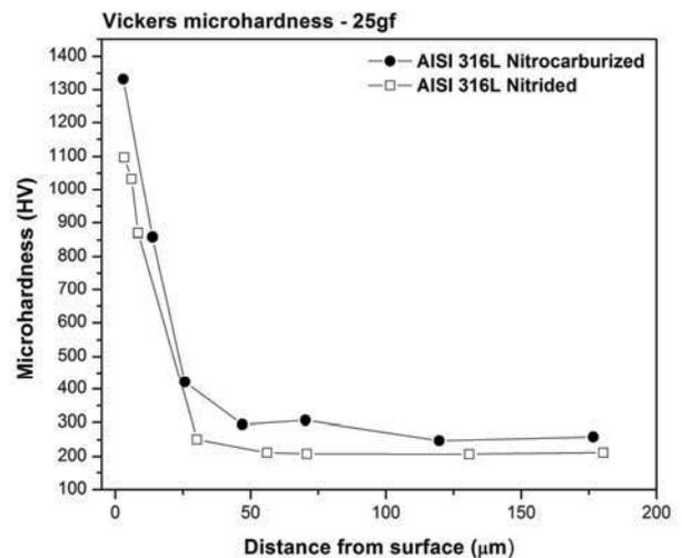
Fig. 3. Microhardness profiles obtained for plasma nitrided and nitrocarburized AISI 316 stainless steel
