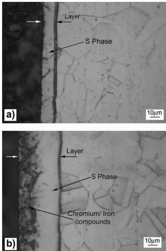
Fig. 1. Optical microscopy of: (a) nitrided and (b) nitrocarburized, AISI 316L
